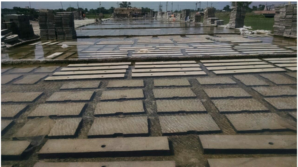
Figure 10 Slabs being cured at Katahari Yard
