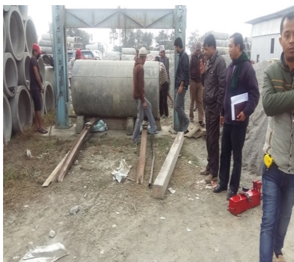
Three Edge Bearing Test of RCC Hume Pipes at Itahari
