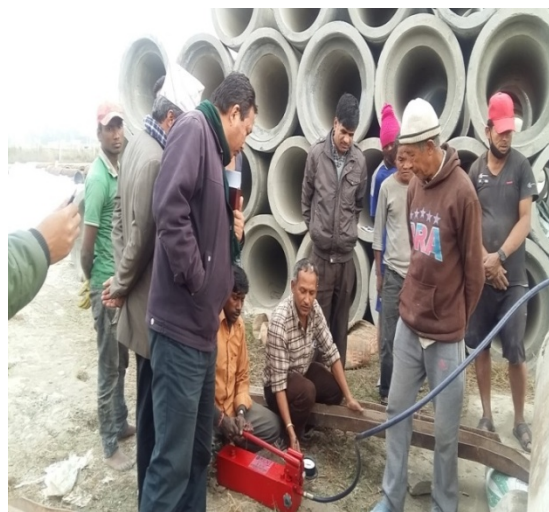
Three Edge Bearing Test of RCC Hume Pipes at Itahari
