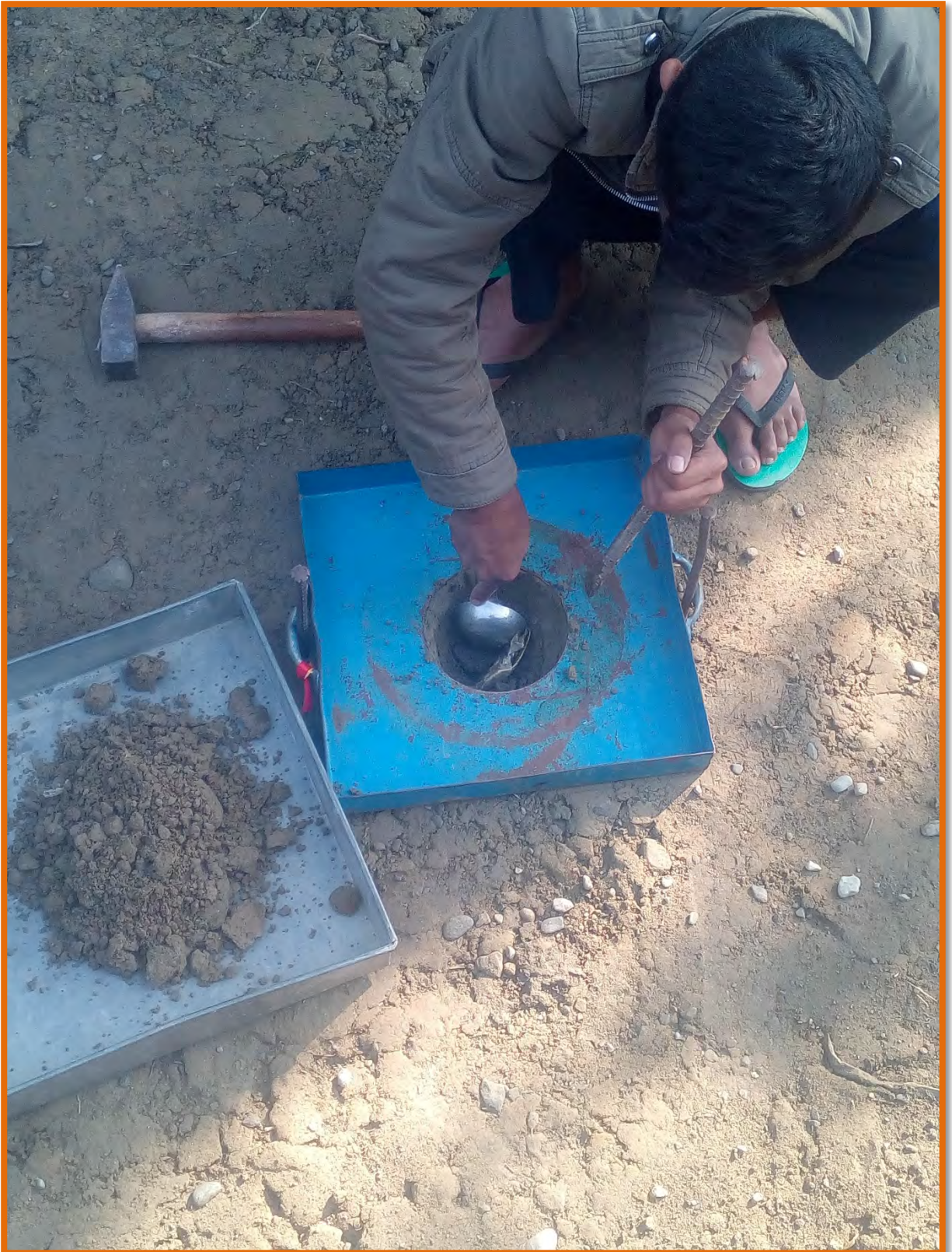
Density test in foundation at R3 road
