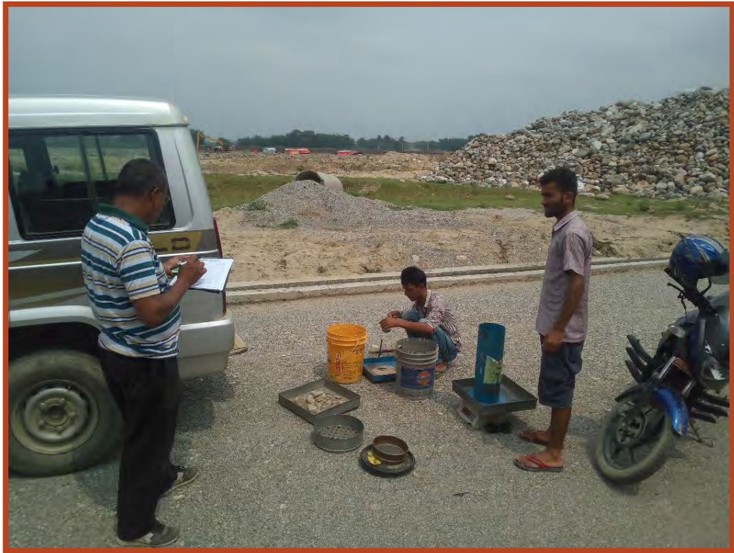
Field Density Test – WWTP's inside road sub base
