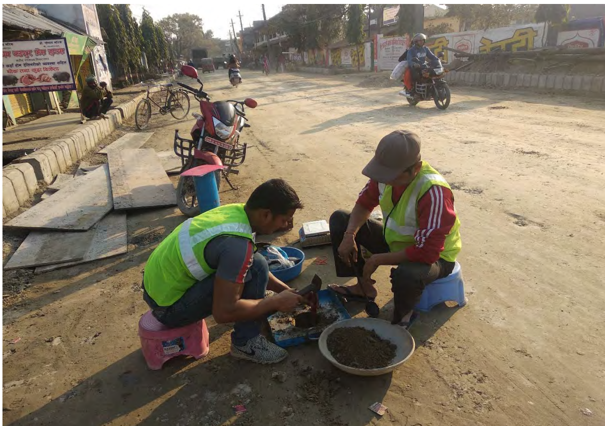
Field Density Test at T3L6 – Moti Marga
